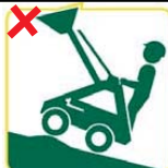
Figure 2 When on a slope, a bump under the front wheels or a hole under the back wheels will increase the angle of the loader and will transfer the weight towards the rear wheels. This may be sufficient to destabilize or tip the loader when at this excessive angle.
