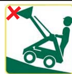
Figure 4 When moving from a shallow incline to a steeper one (up or down), the operator may underestimate the final angle destabilizing or tipping the loader.
