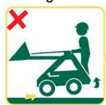
Figure 6 Operating forward/reverse wheel controls suddenly may cause the loader to behave erratically even on flat ground. On sloping ground, any sudden lifting of one end of the machine may cause it to become unstable or overturn.
