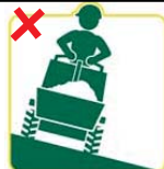
Figure 3 Movement across slopes increases the chances of tipping sideways. The angle of a slope may be difficult to find out unless it is measured.
