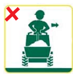
Figure 7 Where the control of one side is released suddenly whilst the other side is still held, the wheels of the released side will stop suddenly causing the loader to change directions quickly and the operator to become unbalanced and may be thrown towards the moving side.
