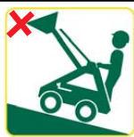
Figure 1 The weight of an operator may cause the front wheels to lift in some situations. Raising the load on an up-slope transfers the weight of the loader back towards the rear wheels. Raising the load fully and/or the operator on the back may cause the front wheels to lift.
