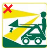
Figure 5 When moving onto a slope from flat ground, the operator will have to lift the bucket so that it doesn't dig in. The extent the bucket needs to be lifted will be difficult to determine and may be more than the safe maximum allowed when all wheels are on the slope.
