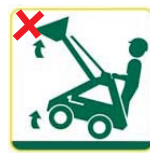
Figure 8 Sudden stopping of upward bucket movement can make the loader buck and on a slope this movement can be enough to overturn the loader.
